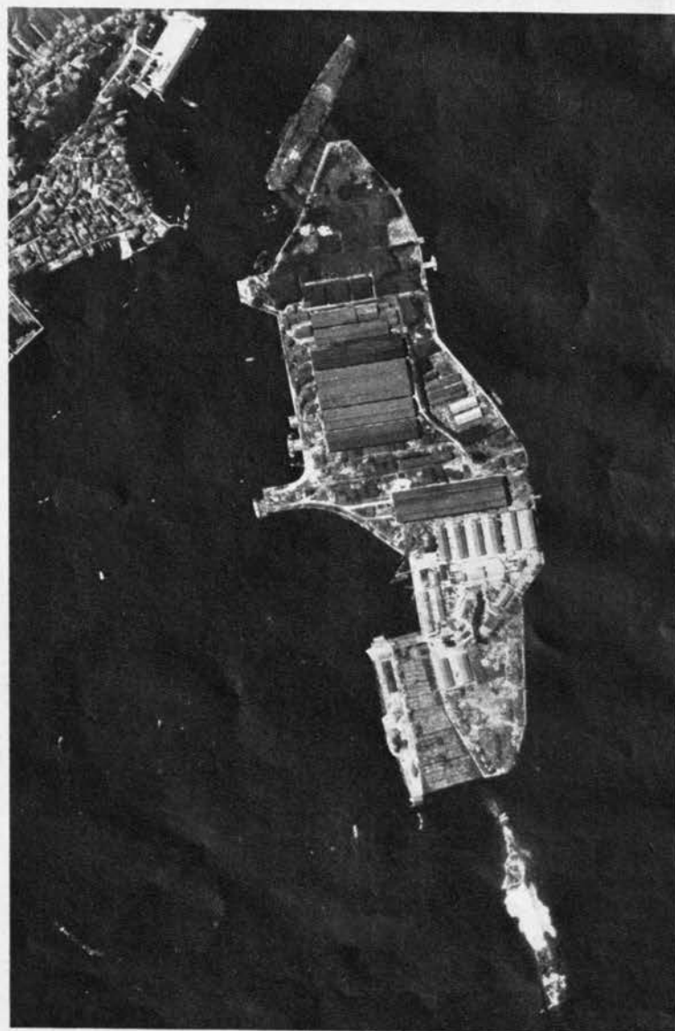
Two Unryu Class CV's are grafted onto an island by nets and deck camouflage. Nets on lower carrier are supported by mass of sampans.
